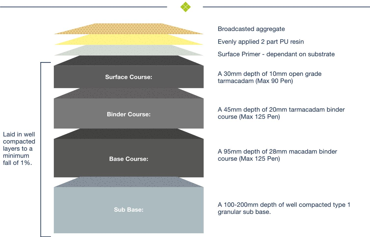
**Allow newly laid surfaces to settle and oxidise for 30 days before applying DekorGrip**
