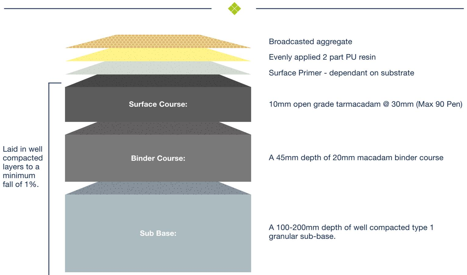
**Allow newly laid surfaces to settle and oxidise for 30 days before applying DekorGrip**
